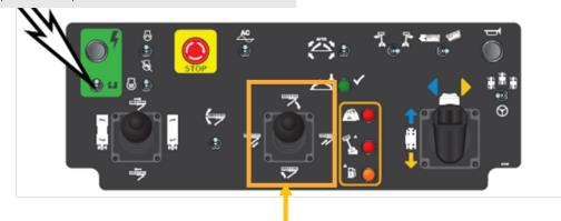
Boom extent/retract and boom lift/ lower function switches
